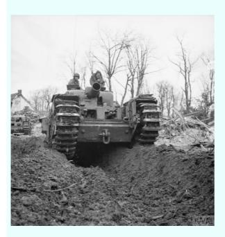
A Churchill AVRE tank with petard spigot mortar could fire 40lb high explosive bombs to destroy concrete fortifications, such as pill boxes and bunkers. They were used at the Normandy Landings on D-Day and after.
